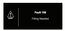
The system may be restarted, re-balancing the water pressure, by using the filling procedure - **see note 1**.
